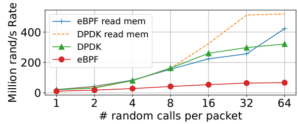
Figure 5: eBPF and DPDK performance when generating different number of random 32-bit numbers per packet using the same prand_u32 function. The eBPF/DPDK read mem plot indicate the performance when reading pre-generated random bits from memory.
